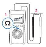
The open terminal voltage is approx. 2.0 V or less. The measurement current (DC) varies depending on the range. To avoid damage to the measurement object, check the specifications before use.
