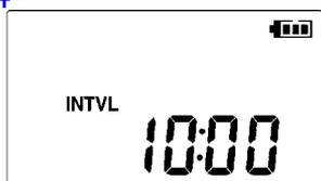
4 Select the recording interval for the logger (in this case, 10 minutes).
