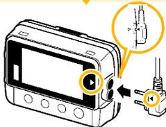
2 Connect the LR9504 Humidity Sensor to the logger.
