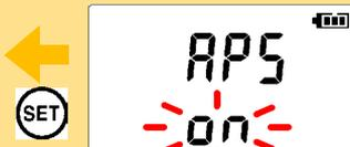
Battery life is extended when on (enabled). (Default is on.)
