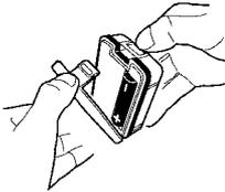
1 Install the battery in the logger.
