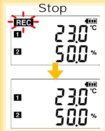
**Stop** Hold the **REC/STOP** button for two seconds while recording (while **[REC]** is displayed).
