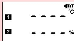
If values are not displayed correctly even when the plug is inserted properly, the logger or sensor may be damaged. Repair may be necessary.
