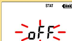
When on (statistical recording), instantaneous, maximum, minimum, and average values are recorded at each interval. Battery life is shorter. (Default is off.) (Record instantaneous values)
