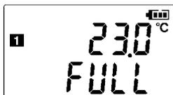
(the Measurement display shows channel measurement value and recorded data count)
